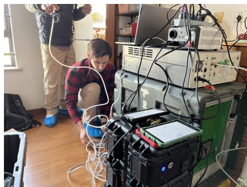
Photo 6 Measuring pollutant emissions in a kitchen in Shanghai
