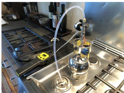
Photo 5 Collecting natural gas from a stove
